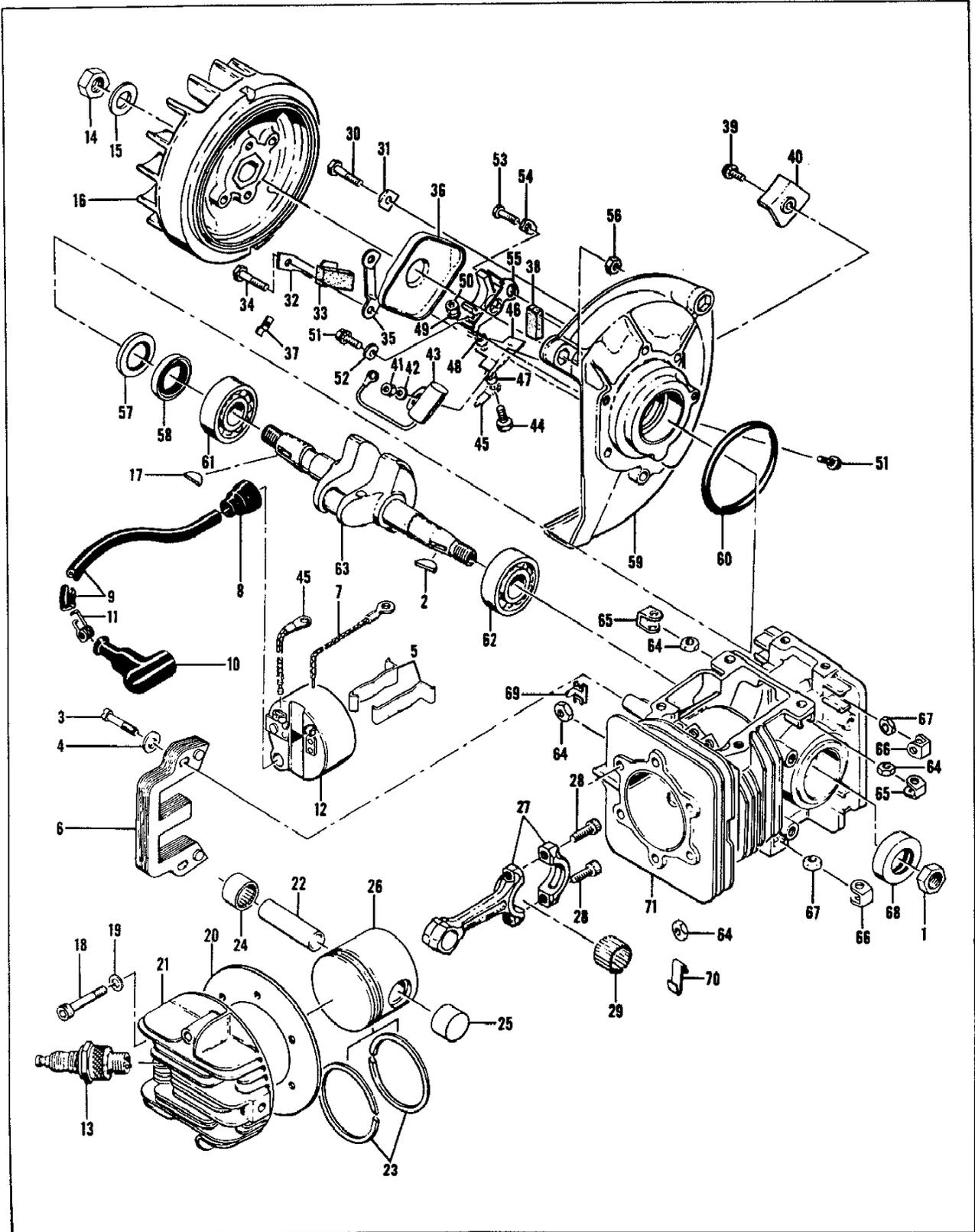
Figure 3. Powerhead Assembly
