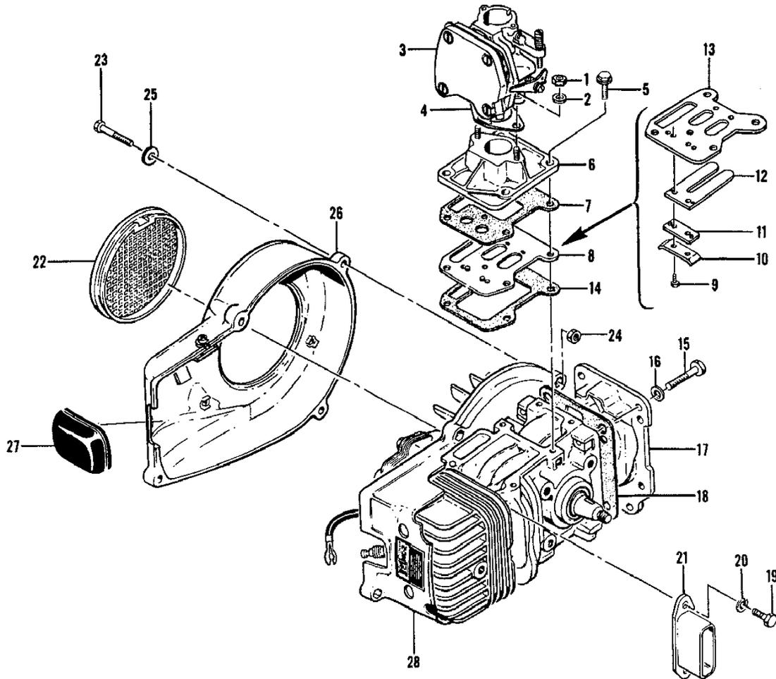
Figure 1. Engine Assembly, Model MC-2 Engine
