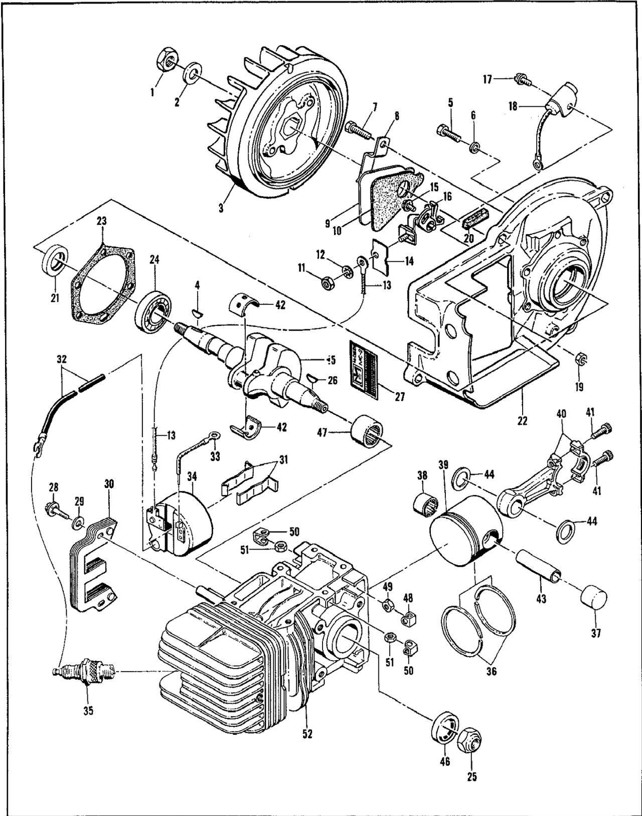
Figure 3. Powerhead Assembly
