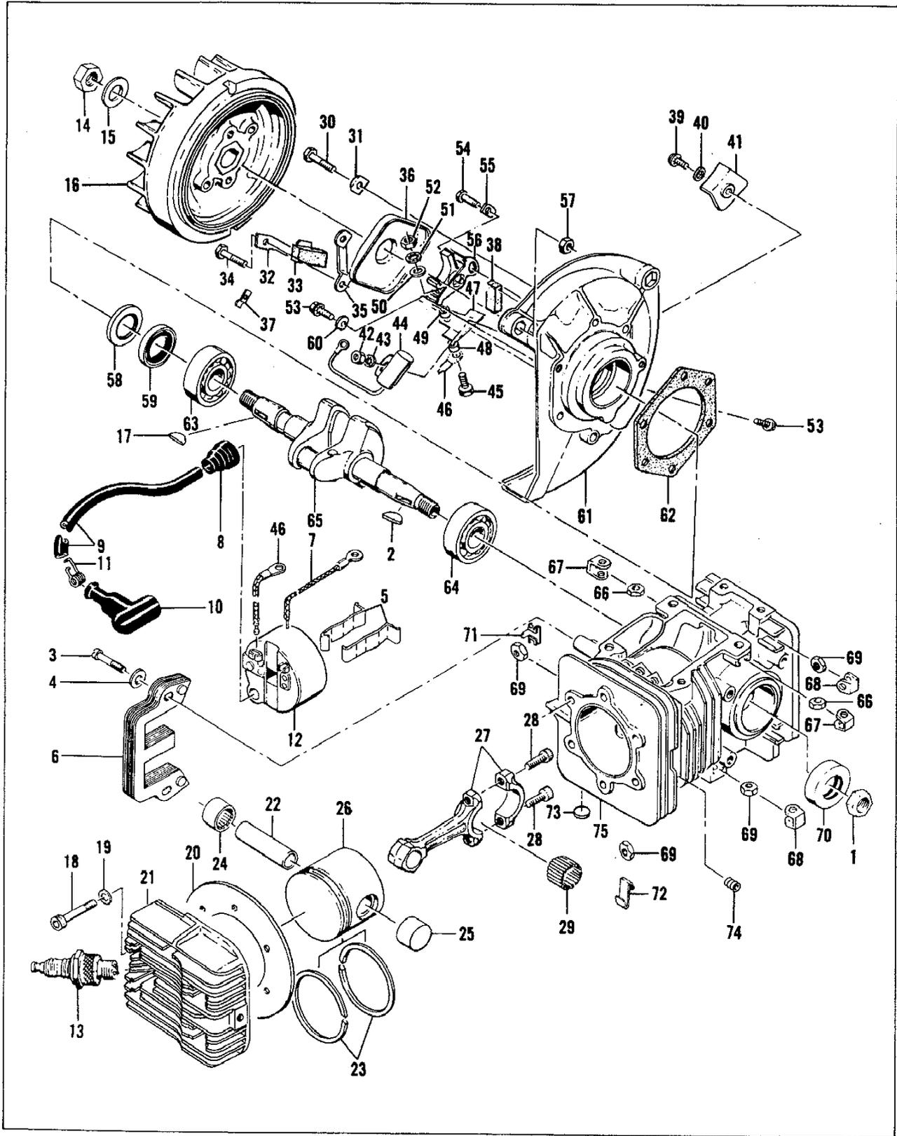
Figure 3. Powerhead Assembly
