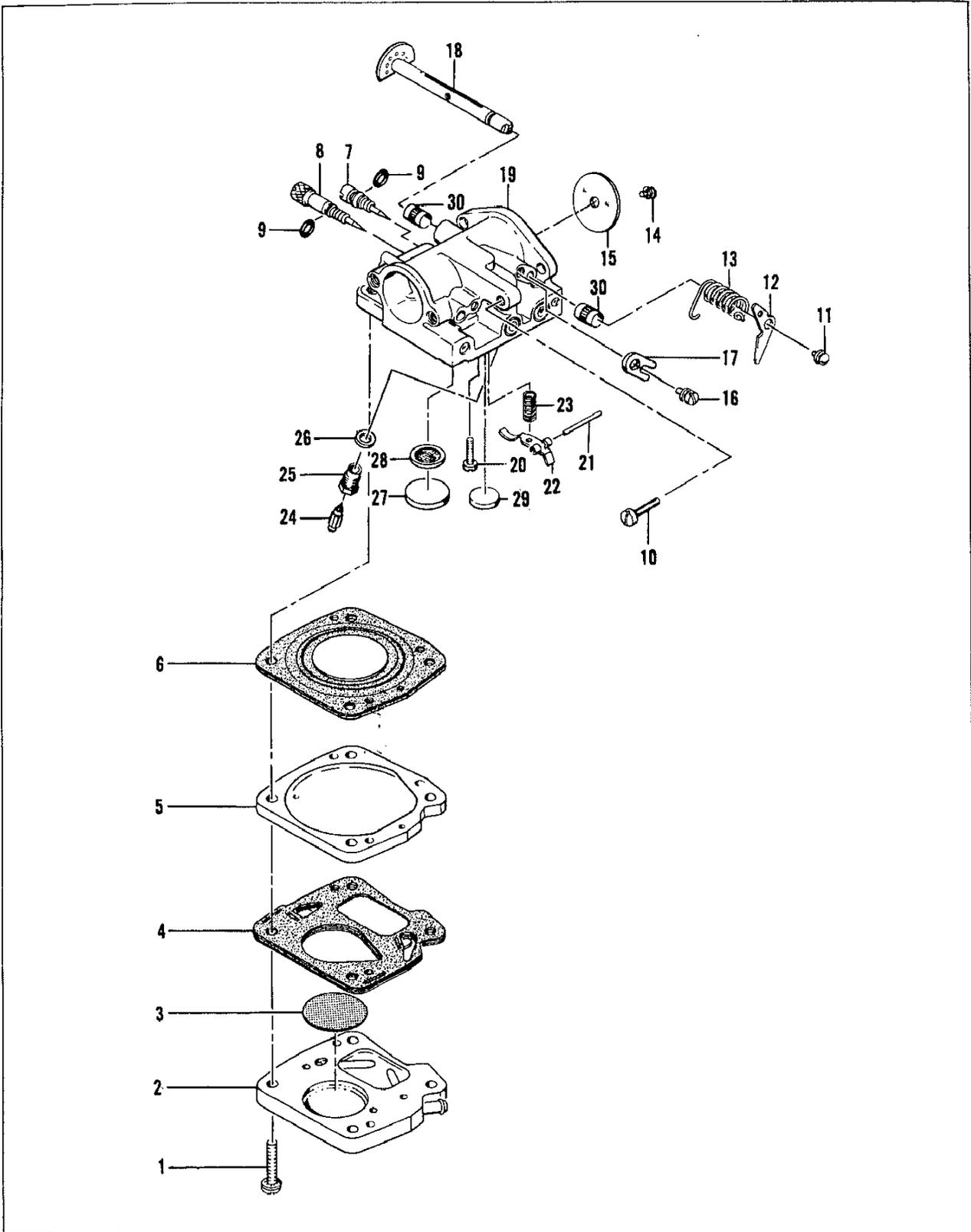
Figure 2. Carburetor Assembly
