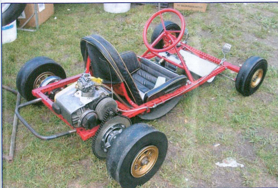
SAE/McCulloch with weight saving holes from a time before minimum weight limits
